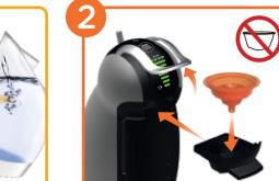
Raise locking handle. Make sure rinsing tool is in capsule holder and capsule holder is in machine. Lower locking handle to close tightly.
